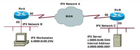
If the configuration to the right is applied to RtrB, the SAP from the IPX server will never be accepted. The result is that RtrA will never notify the workstation of the server's existence. access-list 1000 deny d. 0000. 0000. 0001 access-list 1000 permit -1 interface ethernet 0 ipx network c ipx input-sap-filter 1000
